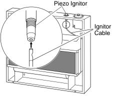
Figure 3 - Attaching Ignitor Cable to Piezo Ignitor
